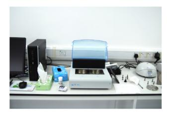
PAS can offer innovative analysis via a new instrument called an 'Oxitest' that measures resistance to oxidative rancidity under accelerated conditions at 90°C and elevated pressure in an oxygen atmosphere. The instrument measures an 'Induction period' (the time taken for antioxidant protection to fail and oxidation to accelerate) and this is a very useful for comparing the potential shelf-life of samples.
